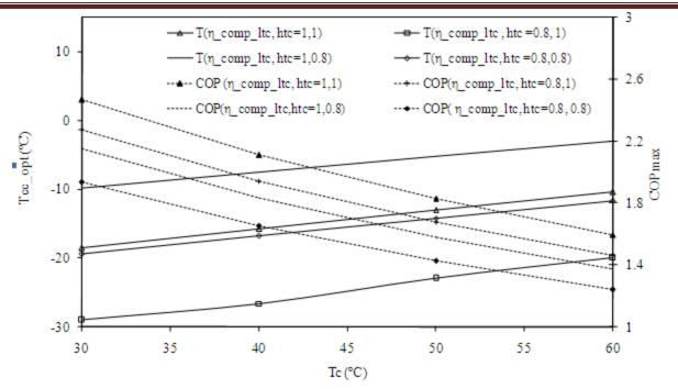
Fig. 8: Condenser temperature versus optimum temperature in cascade condenser and maximum COP for  $R717/R744\,(A=0,\,Te=-45^\circ C)$
