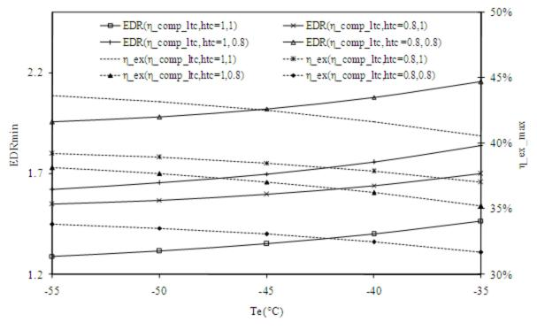
Fig. 7: Evaporator temperature vs maximum exergetic efficiency and minimum EDR for R1270/R744 (A=0, Tc=  $50^{\circ}$ C)
