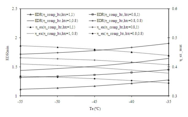
Fig. 5: Evaporator temperature versus maximum exergetic efficiency and minimum EDR for R717/ R744 (A=0, Tc=50°C)
