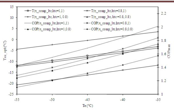
Fig. 6: Evaporator temperature versus optimum temperature in cas cade condesner for R1270/R744 (A=0, Tc= 50°C)
