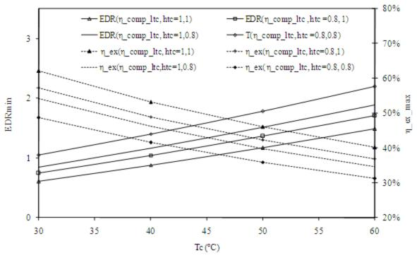
Fig. 9: Condensertemperature versus  $\eta\_ex\_max$  and minimum EDR for R717/ R744 (A=0, Te= -45°C, Tr = Te + 10°C)
