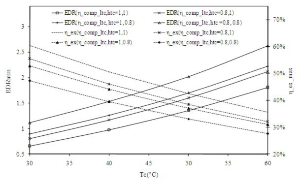
Fig. 11: Condenser temperature versus maximum exergetic efficiency and EDRmin for  $R1270/R744\,(A=0,\,Te=-45\,^\circ C)$
