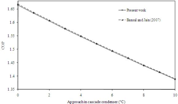
Fig. 2(a) : Approach in cascade condenser vs COP (Comparison of present work with Bansal and Jain[12])- (R-717 in high temperature circuit and R-744 in low temperature circuit) (Te =  $45 \degree$ C, Tc =  $30 \degree$ C, Tcc=  $-15 \degree$ C)
