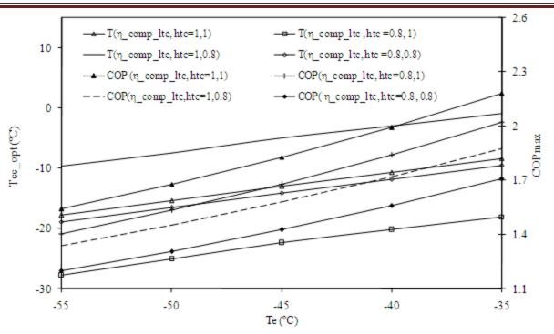
Fig. 4: Evap orator temperature versus optimum temperature in cascade condenser and maximum COP for R717/R744 (A=0, Tc=50°C)
