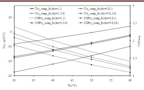
Fig. 10: Condenser temperature vs op timum temperature in cascade condesner and COPmax for R1270/R744 (A=0, Te = -45°C, Tr = Te + 10°C)
